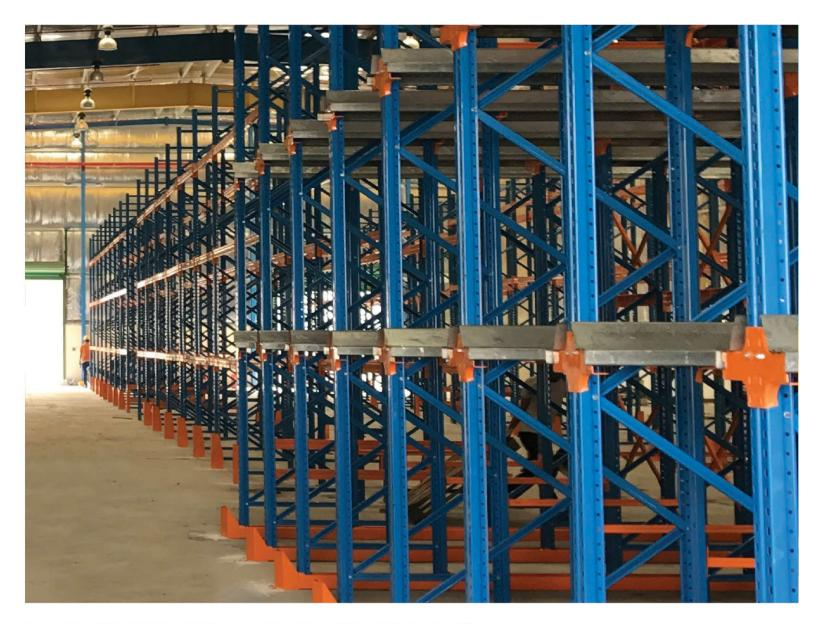
Drive-in racking is designed for the storage of homogenous products. It accommodates a large number of pallets for each SKU. This system makes better use of the available surface and height space than anyother.
